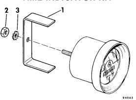
SD0163 QTY REF PART PER NAME OF PART NO NO ASSY \* TIME INDICATOR KIT 173516 1 1 123510 BRACKET 1 204046 2 NUT 1 LOCKWASHER 3 303916 1 \* Not Shown
