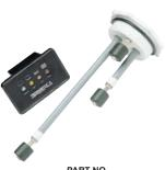
Micro float switches indicate empty, low, mid and full. One light only will indicate at a time to eliminate confusion. No electrical components come in contact with waste or water. Operates on 12 or 24VDC. Can be used for fresh, grey, or black water. Includes probe cap with three micro float switches with 5/8" vent hose connection, indicator panel, gasket, and stainless steel mounting hardware.
