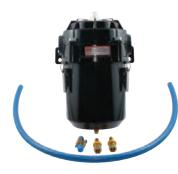
The Racor Crankcase Ventilation Filter will prevent the clogging of engine intake filters, turbo chargers, and intercoolers which will increase performance and efficiency by trapping the oily mist from crankcase blow-by. It will also keep the engine compartment and components clean and reduce environmental pollution, when installed as a closed system. Pop up style indicator alerts need for a filter change.
