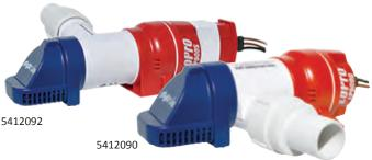
Rule's LoPro Series Bilge Pumps are only 2.4" high. The LP900S model features two automated modes. The first one engages the pump when the water level reaches 2" or 1.3" (user choice); and the second one checks for water by briefly turning on the pump every 2.5 minutes. The LP900D model uses a traditional float and/or panel switch for operation. The entire body swivels up to 180°, making the pump extremely easy to install.
