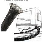
Flex sleeve is a lightweight jacketing for bundling and protecting wires, cables and hoses. Braided from high temperature yarns, this flex sleeve offers total protection for wire and cable assemblies. The unique expansion characteristics make this flex sleeve easy to slip on. Only a few sizes are needed to cover a large diameter range, since each size expands up to four times its normal size.
