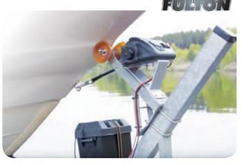
These rugged Fulton XLT Powered Trailer Winches are designed with a 3-position guide to keep the strap straight. The rugged 2" x 15' strap has a 360° swivel hook to prevent twisting.
