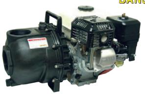
Reliable Honda GX160 will supply the 2" pump with 5.5 HP to give you maximum GPM, and the Honda GX200, will supply the 3" pump with 6.5 HP to give you maximum GPM. Both of these Honda engines are 4 stroke engines with O.H.V. Pull start.
