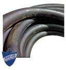
Low Permeation Marine Fuel Hose has a plastic barrier veneer with an NBR outer layer tube to prevent permeation. Polyester reinforced hose complies with EPA and CARB very low permeation requirements and is weather/UV resistant. Primarily used for fuel feed (gasoline up to 85% ethanol blended fuels/diesel/ all bio-diesel blends).
