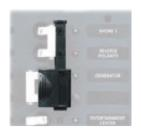
Fits all double pole World or A-Series and Rocker Circuit breakers. Allows only 1 double pole AC Circuit breaker to be activated at a time. Uses circuit breaker mounting screw holes-requires no modification. Includes mounting screws.
