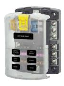
Clear insulating cover with label recess for small format labels. Satisfies ABYC/USCG requirements. Tin plated copper buses and fuse clips give 30A rating for all 12 circuits. Accepts ATO and ATC fast acting blade type fuses. For 12 Circuits.
