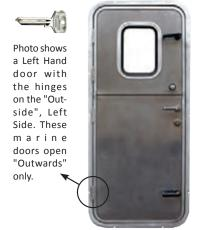
This double panel (Dutch) door is weather tight with gasketed seams, tightening dogs, stainless steel hinges and insulated doubleskinned framed construction. Door comes complete with window, lockset, 2 sets of keys and floating key ring. Framed and pre-hung door is hinged from the left side when viewing from "Outside" your vessel.
