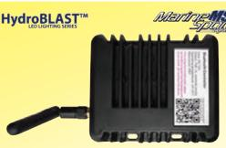
This compact LED Marine Multi-Colour Bluetooth RGB Controller combo gives you convenient control over your marine RGB LED lighting. You can adjust the brightness, colour, fade, flash and more, plus change the look of your system with just the touch of your electronic device. The black box stores neatly in a pocket or cubbyhole. If you can download the app to your cell phone, iPad, or other electronic device, you can control your lights. 1 Year Warranty.
