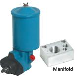
VTM42 Vane pump with **3/4" keyed shaft**. 1/2" ORB pressure port and 5/8" return hose barb. 1000 PSI Relief Clockwise rotation. (Specify if counter clockwise rotation needed).
