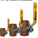
Rated at 600 PSI Designed for water, air & oil. Full flow for a non-restrictive system. Helps prevent cavitation & starvation of pumps.
