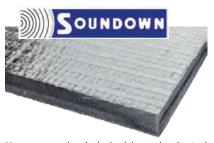
Heavy mass-loaded vinyl layer laminated between two layers of fire-retardant polyether foam covered by an aluminized mylar coating. The easy to clean mylar facing protects the noise dampening foam barriers from spills, mists and vapours.
