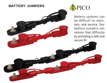
Reducing the amount of exposed connections which in turn reduce the amount of corrosion. Made with 2/0 battery cable, the attached protective caps seal the connection. Fits up to a 3/8" stud.
