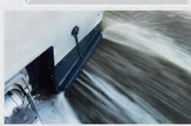
V-shaped interceptors for centerline mounting are perfect for filling the gap between twin outboards or sterndrives, as well as dual propeller tunnels.
