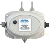
This permanently installed Automatic Outboard Flushing System works whether the vessel is in or out of the water, with the engine off, and in the vertical or tilted position. Water travels from a hose, through the system and is automatically sent to each engine in sequence. The system is permanently plumbed to each engine
