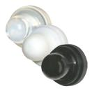
These Push Button Waterproof Boots protect circuit breakers in wet environments. They replace dress nut mounting. For use with push-button, reset-only circuit breakers, 3/8"-27 thread.
