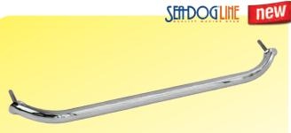
This Stud Mounted Hand Rail is designed to provide a sleek, smooth handrail with no visible mounting hardware. It features integral 5/16"-18 threaded mounting studs. Constructed of corrosion-resistant formed 304 stainless steel. Installs with  $2 \times 5/16$ "-18 nuts (not included).
