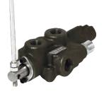
Compact rotary control valve has stainless steel spool. Will operate trap haulers up to 18 GPM flow. 3/4" NPT inlet and outlet, 1/2" NPT pressure ports. Adjustable relief valve is set at 1500 PSI. Max pressure 3000 PSI 18 GPM Max Flow.
