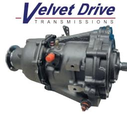
The Velvet Drive "71" and "72" designations indicate input horsepower ranges. The most popular model is the in-line unit. "In-line" indicates that the input and output shafts of the transmission are on the same axis. Direct drive versions of the in-line models are frequently used on high horsepower, light weight boats. The reduction ratio versions use an additional planetary gear set to allow the use of larger propellers for greater pulling power at lower shaft speeds.
