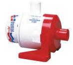
Designed for use as a washdown pump and/or to circulate water to your livewell tank(s). Heavy duty construction for use on commercial or pleasure boats. Because it is a centrifugal pump, it must be located below the water line to ensure prime. Uses 1-1/2" hose.
