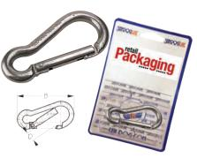
These Snap Hooks feature a key-lock connection for added security. For use with ropes, chains, straps and small diameter cable. Made of formed 316 stainless steel.
