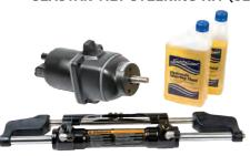
Single and dual non-power-assisted outboard engines up to 350 HP (700 combined HP for counter-rotating duals) that have ABYC standard engine tilt tube. Ideal for cruisers, runabouts, center console boats, offshore fishing boats and many more. Suitable for speeds up to 60 MPH and dual station use (with purchase of extra helm, hose and fittings). Allows independent engine tilt in dual engine installations. Dual engines require purchase of a tie bar kit and extra hardware.
