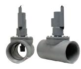
The Aqualarm Cooling Water Flow Detector Monitors Marine Engine Raw Water Flow to prevent engine damage due to overheating. It will activate a visual or audible device (not included) immediately whenever raw water flow slows to below 6-8 GPM.
