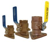
Full flow flange valve provides an unrestricted flow for engines and pumps. Stainless Steel lever and nut with all bronze wetted metallic components. No lubrication required, PTFE seats and seals. Winterizing drain plug and bonding screw are standard.
