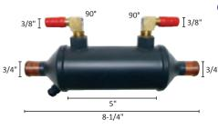
8-1/4" **Total Length: Body Length:** 5" Water Connection: 3/4" Oil Connection: 3/8", 90°
