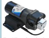
This Constant Flow Water Pressure Pump has an electronic control system that operates a variable speed drive. This enables the motor to speed up or slow down and match the water demand in real time providing consistent high pressure for up to 4 faucet/shower combinations simultaneously.
