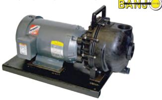
Banjo Pump completely assembled with a 5 HP heavy duty Baldor Electric Motor. A polypropylene pump head and PTFE coated internal fasteners provide corrosion resistance. A precision moulded construction with a 1" spacer and a specially designed slinger/shaft seal provide maximum motor protection and low maintenance. Maximum lift of 15', 215 GPM at 3450 RPM.
