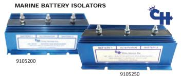
Solid state device allows you to connect your engine alternator directly to both batteries without fear of overcharging, or of one higher-charged battery discharging into the other lower-charged battery. For 6, 12, 24, 32V negative ground systems with one alternator and two batteries. 5/16" posts.
