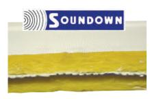
Heavy lead laminated between two layers of fiberglass produce a fireproof noise barrier that is Coast Guard Approved. White coating protects against absorbing fumes and oils.
