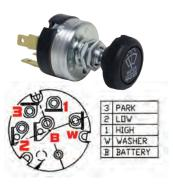
2 Speed Wiper/Washer Switch with push knob washer control and copper alloy blade contacts 12VDC, 24VDC and 32VDC
