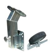
This Angled/Pivoting Spare Tire Carrier allows your spare tire to fit at an angle under the bow of the boat. It is adjustable to fit 4, 5 and 6 lug wheels. The unique pivoting feature allows the tire to swing down for easy loading or removal of your spare. The carrier comes with three sets of U-Bolts to fit trailers with 3", 4" and 5" frame tubes.
