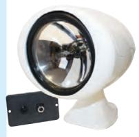
Sweeping curves complement the latest Pleasure Craft profiles. Finger tip control of the water tight halogen sealed beam will pick out hazards nearly 900' away. Easily replaceable 5" halogen seal beam delivers 100.000 candle power. Comes complete with joystick remote control, plastic housing and base. Comes with 15' cable. Full 320° horizontal rotation, 75° vertical sweep.
