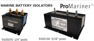
Solid state device allows you to connect your engine alternator directly to both batteries without fear of overcharging, or of one higher-charged battery discharging into the other lower-charged battery. Batteries are electrically isolated from each other. For 6, 12, 24, 32V negative ground systems with one alternator and two batteries.
