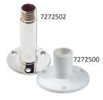
Shakespeare flange mounts can be used to attach marine antennas to deck or bulkhead. The mounts do not adjust for slanted surfaces, and do not allow lowering the antenna for fishing, passage under overhangs, or for boat storage and towing. They are usually used for small antennas, GPS and radar devices, and marine TV antennas atop radar arches etc.
