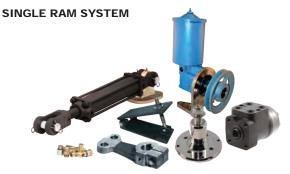
Mermaid's Single Ram System is very rugged and has proven itself to be very reliable. The system includes helm, stainless steel helm plate and steering shaft, 2" bore cylinder, brass cylinder hold down bracket, bronze tiller arm, tiller arm bushing (1-1/4" only), power steering pump with tank, 7" pump pulley, adjustable pump bracket, stainless steel hardware and hose fitting kit.
