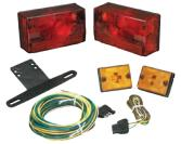
The kit comes complete with two tail lights, two amber clearance/side marker lights with reflex lens, 20' trailer wiring harness cable with moulded four prong plug, 4' four wire car wiring harness cable with moulded 4-way plug plus license plate bracket. Dimensions: 6" x 3-1/2" x 2-1/4"
