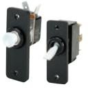
For applications such as starters, bilge pumps, horns, wipers and engine controls where switching, in addition to circuit protection, is required. All panel switches mount in Blue Sea Systems' circuit breaker panels. Supplied with mounting adapter for standard 5/8" circuit breaker mounting hole. Nickel-plated brass and phenolic non-corrosive construction.
