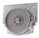
This rugged line of hauler heads are manufactured completely of corrosion proof materials: Aluminum back plate, stainless steel discs, stainless steel hub with grease passage, stainless steel hub cover with grease nipple, stainless steel splitter, stainless steel rope deflector, motor fittings, stainless steel fasteners exclusively. Choice of hydraulic motors (included) are listed below:
