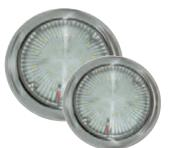
Made of 304 Stainless Steel with a high impact strength Polycarbonate lens, these super slim dome lights are great for surface mounting just about anywhere. As slim as they are, they can provide a lot of light output using many high power LEDs. 12V. LED has a lifetime of 50,000 hours.
