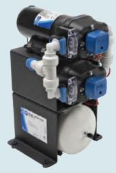
These Xylem Stacked Water Systems are fully assembled water pressure sets which makes installation of water pressure systems simple. Thermal protected pumps are assembled onto a pre-pressurized accumulator tank providing a smooth flow. They are self-priming up to 10' (3m), they have run-dry ability. Complies with ISO 8846 Marine (Ignition Protection)
