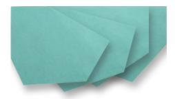
Oilit CAF is a premium grade CAF sheet with a Nitrile/Natural rubber binder. It is designed for high temperature and pressure involving steam, gases, hot oil, fuels, solvents, alkalis, mild acids, gasoline, benzol, ether, ethyl, amyl acetates, glycol, and many other severe applications. Oilit CAF has a temperature limit of 1000°F and maximum pressure of 2000 PSI. Thickness: 1/16"
