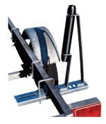
These Roller Guide On's are adjustable to the hull angles. The hot dip galvanized steel base with one piece U-bolt fits all channel and tube frames up to 5" and is adjustable up to 8" per Side for a total of 16" overall.
