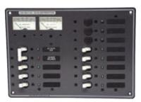
BLUE SEA 13 Breaker position panel with 30A. AC Double pole main breaker and 8 x 15A breakers installed. Red reverse polarity indicating LED & green LED circuit 'on' indicators. Complete with 0-150VAC voltmeter & 0-50A AC ammeter. All hot, neutral & safety ground buses installed and pre-wired.
