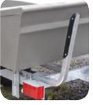
These Low Rider Guide On's are ideal for jon boats, bass boats and personal watercraft. The guide posts are made of 1-1/2" square, 16-gauge steel tubing and galvanized for long life. Guide covers are made from high impact non-marking moulded PVC. They mount to trailer cross members 2" wide by 2"or 3" high. All mounting hardware included.
