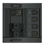
This source selector panel has two 50A Flat Rocker style Main breakers with a lockout slide to prevent from connecting multiple AC Sources simultaneously.
