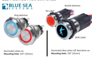
These contemporary and compact Ring and Backlit Push Button Switches have a 316 Stainless Steel housing for optimal appearance and corrosion resistance. An O-ring panel gasket and a moulded rear cover provides an IP67 Waterproof rating. ISO 8846 Marine Ignition Protection.
