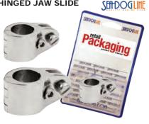
Durable and corrosion resistant with a set screw on the back allows you to quickly and easily adjust the placement of these slides where they are needed. Made of investment cast 316 stainless steel.
