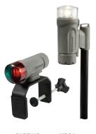
Made of a shock-proof composite material & shatter-proof polycarbonate, They are water-resistant, easy to use, and operate on three AAA batteries (not included) with a typical run time of 150+hours. it includes red/green LED bow light, white LED stern light, quick release heavy-duty mounts, pole, and hardware. These lights are not intended to meet Transport Canada regulations. Not meant for use on boats that can exceed speeds of seven knots.
