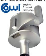
These Residential Grade compact spiral chambered mufflers have an all MIG welded construction. They have a steel wool and mesh liner providing premium silencing with low back pressure. The connections are standard Slip-Fit. These models are available in a Carbon Steel with a high-temperature black finish or 316 Stainless Steel.
