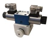
Also called 'Auto Pilot Valve'. This unit is solenoid operated and flow control from 0.5 to 12 GPM to control rudder speed. This system is usually used with auto pilot and/or joy stick installation.
