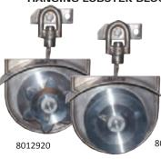
This unit has a S/S frame with a 7" aluminum star or blank pattern wheel. Manufactured with a rugged swivel neck, bronze bushings, stainless steel grease nipples, stainless steel guard, and back shield.
