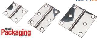
These Stainless Steel butt hinges are designed for a flush installation. Installs with four #8 FH fasteners (not included). Made of stamped stainless steel.
