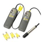
Track and trace open and short circuits, broken wires and current leaks. No wire piercing is required; this non-contact system will trace hidden wires inside bundles, harnesses, conduits and/or behind panels. A variable audio/visual signal will provide fast and intuitive feedback on circuit/wire proximity. Adjustable sensitivity for all tracing situations. The Transmitter has auto polarity. Compatible with 6 to 42VDC circuits.
