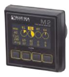
The M2 OLED Digital Bilge Monitor has a bright, waterproof, daylight readable OLED display to indicates if a bilge pump is on, how long it has run in the last hour, and shows a cycle count. The M2 monitor provides an average cycle count over a typical 24 hour period for quick indication of a potential problem. Monitors up to four bilge pumps.
