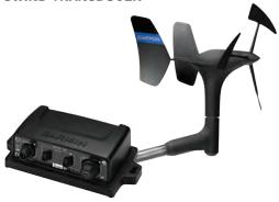
The gWind transducer features twin-fin technology with 3-bladed propeller for more accurate TWS in lighter air while the twin-fin design gives a more stable TWA. The 3-bladed propeller, unlike a cups design, is always efficient. Combined with optic reading, this transducer provides superior accuracy at low wind speeds and also provides for excellent linearity.
