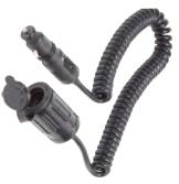
This Extension is designed to withstand the rigors of wet environments and constant vibration. The Plug features an "ON" indicating LED, a moisture proof sealing ring around the shaft, a strain relief, and a built-in 10A fuse. The Socket features a watertight cap, easy installation and interlocks with the plug. A Twist Lock System allows the plug to lock securely into socket.
