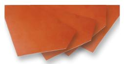
Albion 300 is made from an SBR compound resulting in a sheet soft enough to make a tight fluid seal, strong enough to resist a blow-out. It is suitable for use against hot or cold water, air and low pressure steam. Albion 300 has a 225°F temperature limit and exceeds ASTM D 1330-78 Grade II. Available in two thicknesses. Available in 48" x 48" sheets or per square foot. Minimum order of 12" x 48"
