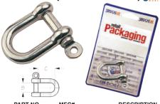
Straight sides with a U-shape rounded end, Designed for rigging applications with bi-directional loads. Made of investment cast 316 stainless steel. Cast shackles are not load rated.
