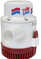
3700 GPH Pump. Heavy duty construction for both commercial and pleasure boat use. Ignition protected, double insulated. Permanently lubricated "Ball Bearing" motor. Water cooled motor for longer life. No burn-out when run dry. Uses 1-1/2" hose.
