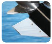
The Megaware KeelGuard provides the best of two worlds. It will protect and prevent damage to your motor's skeg and can also be used to repair and replace an already broken skeg.
