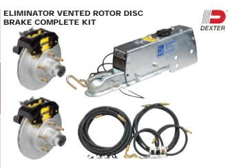
Kit comes with everything needed to replace trailer disc brakes for faster stopping power. New model 660/800 disc brake actuator features a cast ball clamp, Drop N Go auto coupler latch, oversized master cylinder, with back flow style solenoid installed. Includes a pair of GalvX coated vented rotor disc brakes, Aluminum calipers, disc brake actuator and brake line kit. Also includes brake hoses, brass fittings and attachment hardware.
