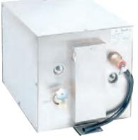
These water heaters feature aluminium tanks and hold down brackets, dual wall heat exchangers, and ignition protection with your choice of marine galvanized or stainless steel exteriors.
