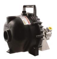
Gresen MGG2 hydraulic motor driven pump provides a minimum 6 GPM, and a maximum 10 GPM with a minimum 200 PSI and a maximum of 2000 PSI Pump has a maximum RPM of 3600. The hydraulic motor has a built-in adjustable bypass valve. Open or closed system.
