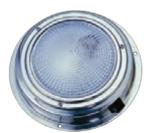
This surface mount LED Dome light has a Stainless Steel housing containing 20 x 0.2W Natural White LEDs with a beam angle of 120°.
