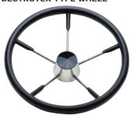
Deep dish with 25° spoke angle. Constructed of high grade nonmagnetic stainless steel, these wheels have a cast and welded hub and welded spokes at the rim. Covered with quality foam at the rim for better grip and warmth. 3/4" tapered bore. 2-1/2" black center cap.
