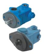
Hydraulic vane pump with internal flow control valve for power steering applications. 1" FPT inlet port, 1/2" ORB pressure port and 1/2" FPT return port.
